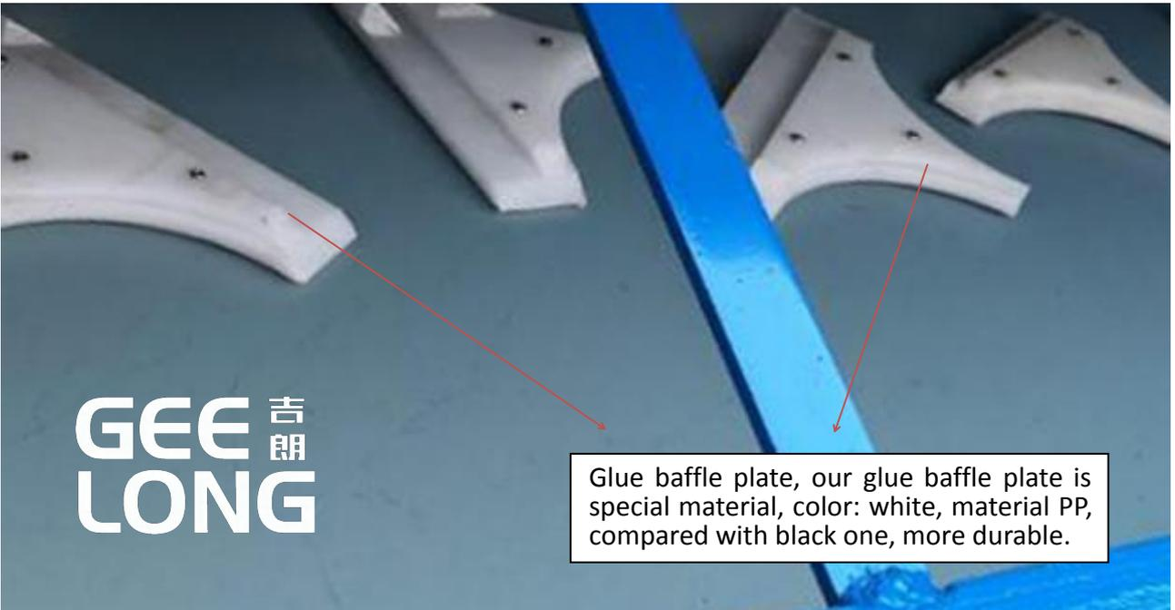
Glue baffle plate, our glue baffle plate is special material, color: white, material PP, compared with black one, more durable.
