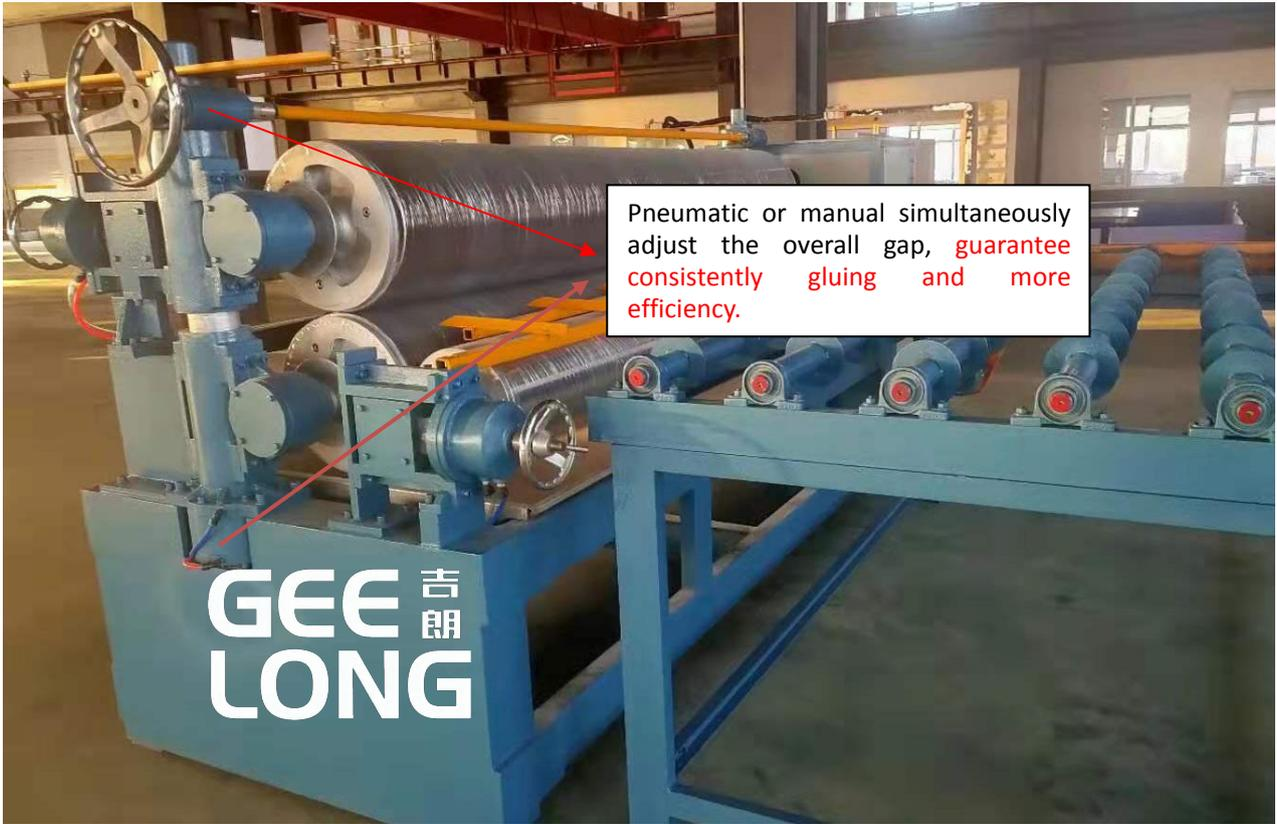
Pneumatic or manual simultaneously adjust the overall gap, guarantee consistently gluing and more efficiency.
